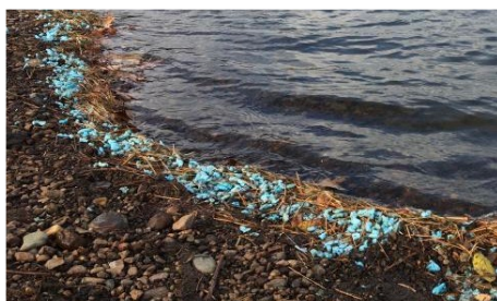
Images of unencapsulated polystyrene, from broken dock floats, in various states of decay.
